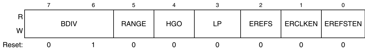
Figure 11-4. ICS Control Register 2 (ICSC2)
