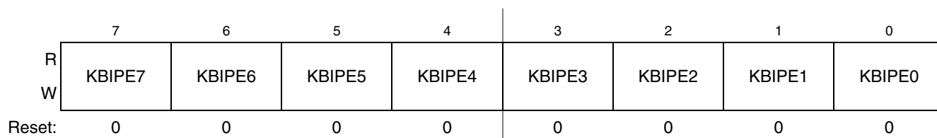
Figure 7-4. KBI Interrupt Pin Select Register (KBIXPE)
