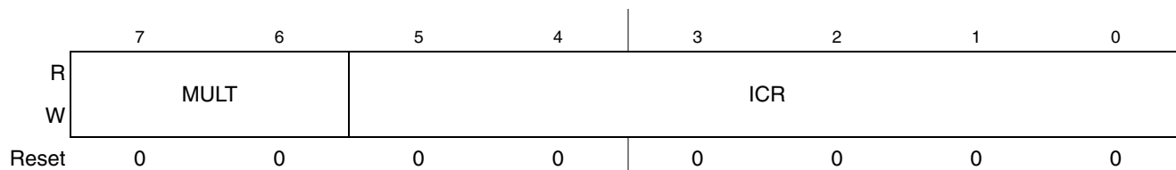
Figure 12-4. IIC Frequency Divider Register (IICF)
