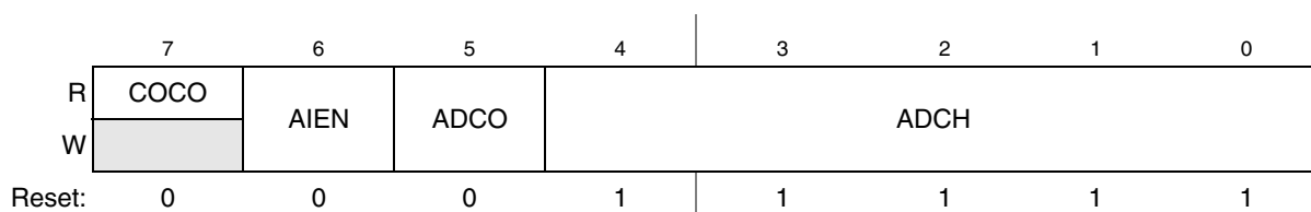
Figure 10-3. Status and Control Register (ADCSC1)
