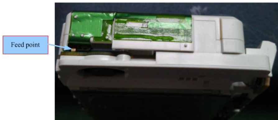
Figure 6: Example of FPC Monopole Antenna
