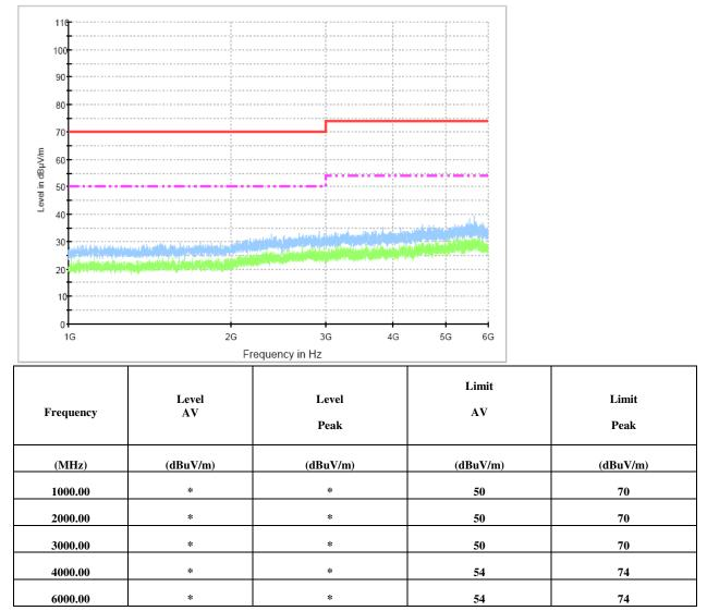
""" means the emission level is 6dB lower than the relevant limit.
