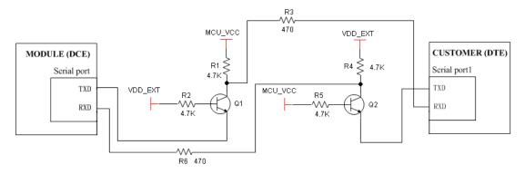
Figure 4: The lever shifter by transistor for communication with MCU
