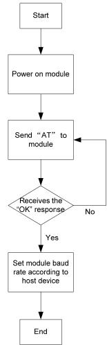
Figure 6: Synchronizing baud rate flow chart
