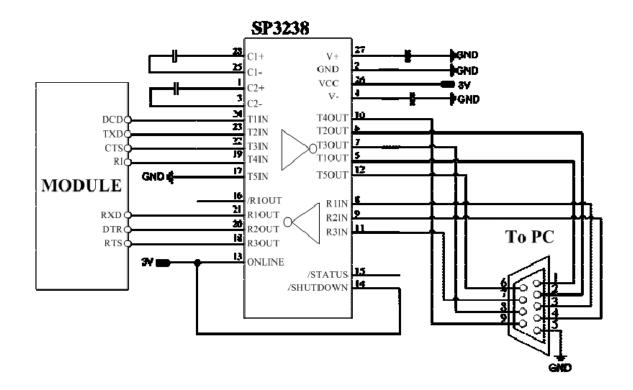
Figure 5: The lever shifter by SP3238E for communication with PC 7 SIM900\_Serial Port\_Applocation Note\_V1.03
