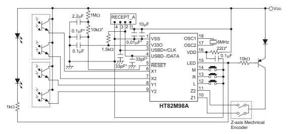
Note: Layout 0.1μF capacitor, 22Ω resistor and 0.01μF capacitor as close to VDD pin as possible.
