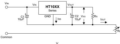
$$I_{OUT} = \frac{V_{XX}}{R_{A}} + I_{SS}$$
