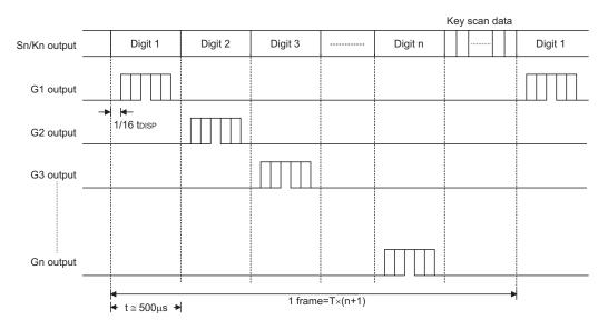
Note: One cycle of key scan consists of two frames, and data of 12×4 matrixes is stored in RAM.
