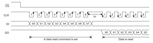
DO must be sure to connect an external pull-high resistor to this pin (1k $\Omega$  to 10k $\Omega$ ).
