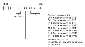
Note: power-on status: 1-16 pulse width is set and the display is turned off. Key scanning will be stopped during power
