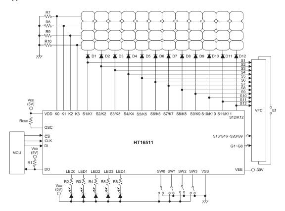
Note:  $R_{OSC}$ =51k $\Omega$  for oscillator resistor
