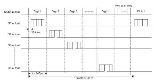
Note: One cycle of key scanning consists of two frames, and data of 16×2 matrixes is stored in the RAM.
