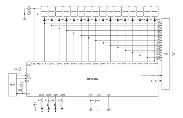
Note:  $R_{OSC}$ =82k $\Omega$  for oscillator resistor R1=1~10k $\Omega$  for external pull-high resistor R2~R6=750 $\Omega$ ~1.2k $\Omega$ R7~R8=10k $\Omega$  for external pull-low resistor D1~D6=1N4001 Ef=Filament voltage for VFD C=0.1 $\mu$ F~1.0 $\mu$ F
