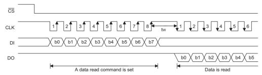
Be sure to connect an external pull-high resistor to this pin (1k $\Omega$  to 10k $\Omega$ ). Note: 1. When data is read, a wait time "t<sub>W</sub>" of 1µs is necessary at 5V.
