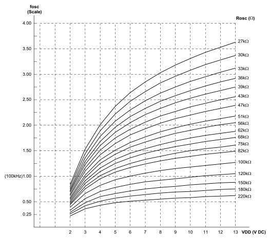
Note: The recommended oscillator frequency is  $f_{OSCD}$  (decoder)  $\cong 50 \; f_{OSCE}$  (HT12E encoder)  $\cong \frac{1}{3} \; f_{OSCE}$  (HT12A encoder).
