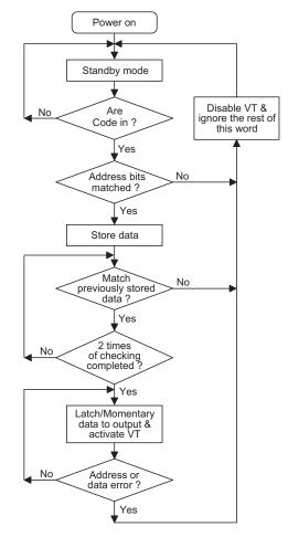
The oscillator is disabled in the standby state and activated as long as a logic "high" signal is applied to the DIN pin. i.e., the DIN pin should be kept "low" if there is no signal input.
