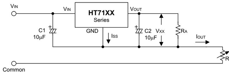
$$I_{OUT} = \frac{V_{XX}}{R_A} + I_{SS}$$
