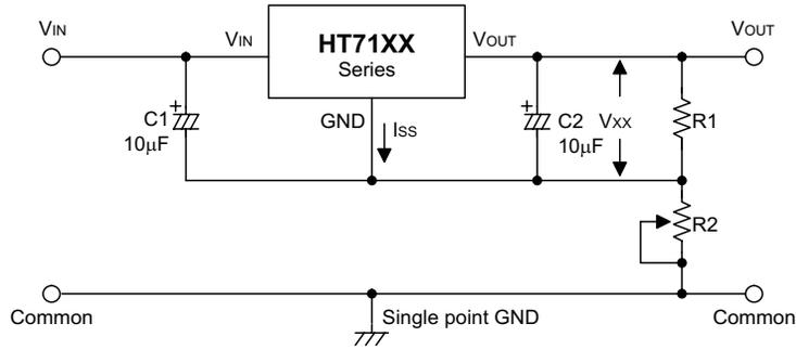
$$V_{OUT} = V_{XX} \left(1 + \frac{R2}{R1}\right) + I_{SS} R2$$
