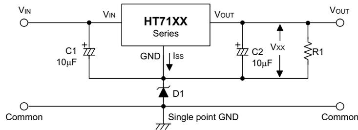
$$V_{OUT} = V_{XX} + V_{D1}$$
