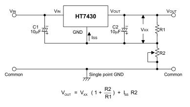
**Circuit for Increasing Output Voltage**
