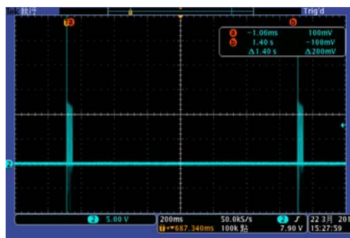
Fig 11 (2). SCP test PWM at 85Vac
