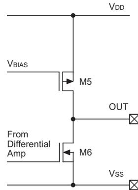
Because of the consideration for minimized power consumption, the output short circuit current is limited to about  $-1.2mA$  for source drive and  $4mA$  for sink drive. This is believed to be enough for most low power systems, however it is recommended to use the load resistor of  $>1M\Omega$  for normal applications. In case of heavy load driving, an external buffer stage using bipolar transistors is recommended.
