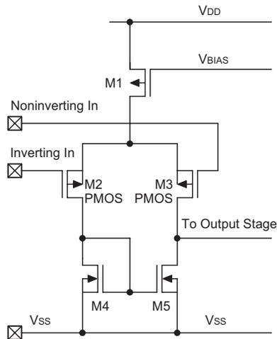
Since the input impedance of PMOS is inherently very high, it can directly couple to high impedance elements without loading effect. For example, coupling to ceramic transducers, integrating capacitor and resistor networks.
