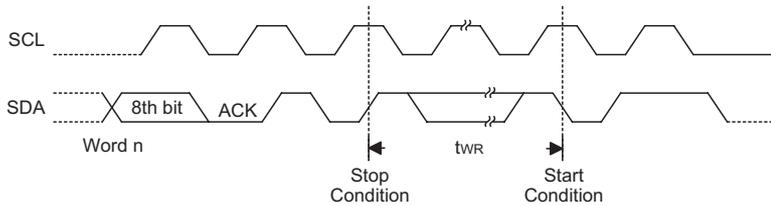
Note: The write cycle time  $t_{WR}$  is the time from a valid stop condition of a write sequence to the end of the valid start condition of sequential command.
