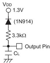
Note: C<sub>L</sub> = 100pF including jig capacitance.
