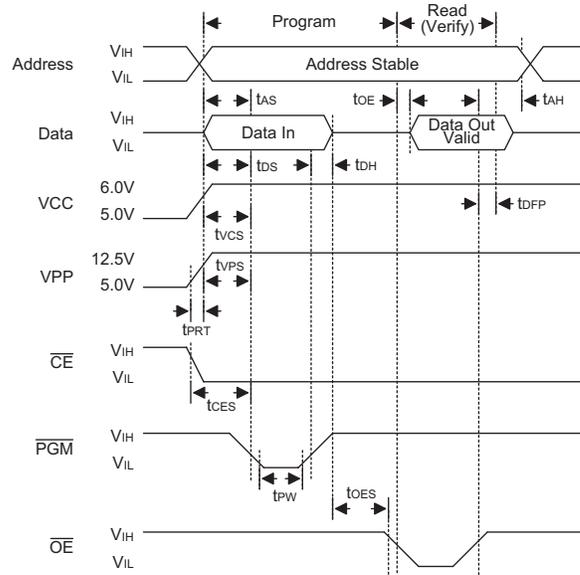
Figure 2. Programming Waveforms
