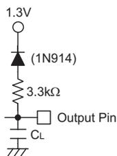
Note: C<sub>L</sub>=100pF including jig capacitance.
