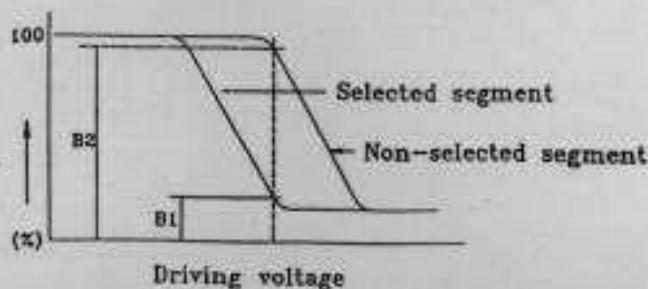
$$K = \frac{\text{Brightness of non-selected segment (B2)}}{\text{Brightness of selected segment (B1)}}$$
