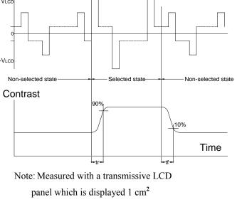
$V_{LCD}$ : Operating voltage  $f_{FRM}$ : Frame frequency : Response time (rise)  $t_f$ : Response time (fall) tr
