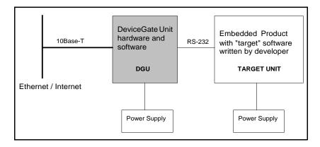
• Ethernet-enabled hardware and software, which is designed to be tightly integrated into a product as a daughter board, with communication via logic-level signals.
