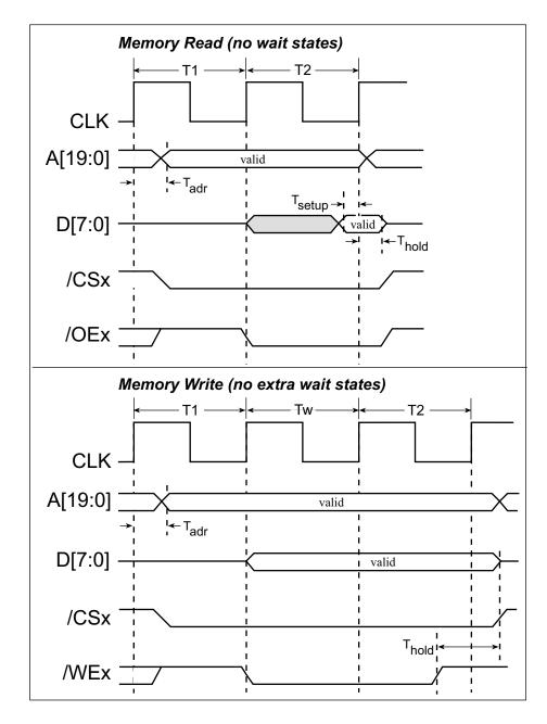
Figure A-4. Memory Read and Write Cycles
