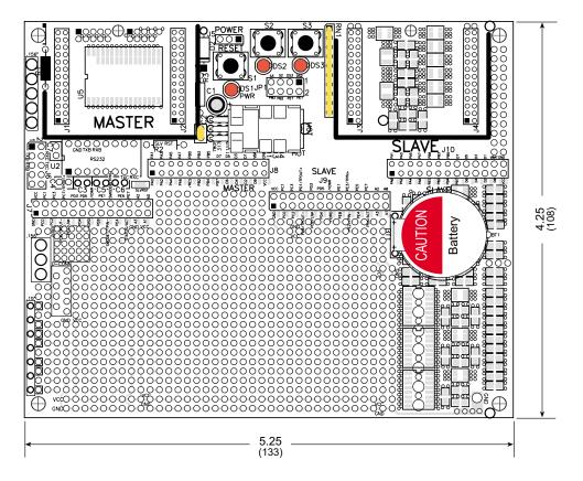
Figure B-1. RCM2200 Prototyping Board Dimensions
