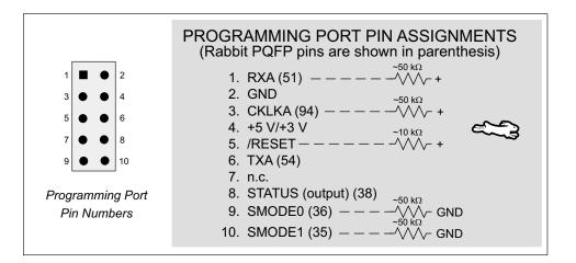
Figure E-1. Programming Port Pin Assignments
