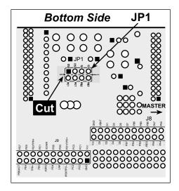
Figure B-3. Where to Cut Traces to Permanently Disable Demonstration Hardware on Prototyping Board
