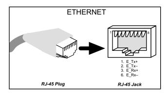
Figure 3. RJ-45 Ethernet Port Pinout
