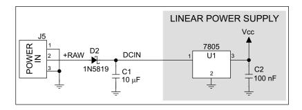
Figure B-2. Prototyping Board Power Supply
