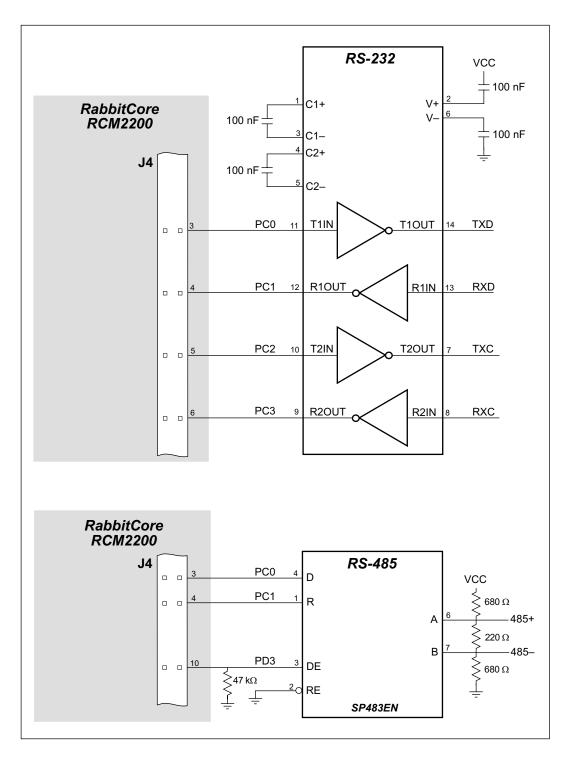
Figure D-1. Sample RS-232 and RS-485 Circuits
