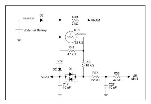
Figure C-2. RCM2200 Battery-Backup Circuit
