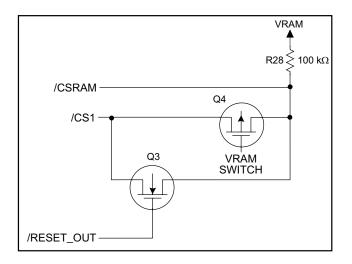
Figure C-3. Chip Select Control Switch
