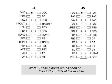
Figure 2. RCM2200 I/O Pinouts
