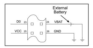
Figure C-1. External Battery Connections at Header J5
