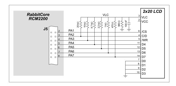
Figure D-3. Sample LCD Connections
