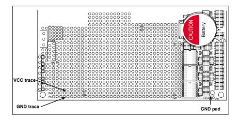
Figure B-5. VCC and GND Traces Along Edge of Prototyping Board
