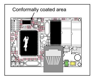
Figure A-6. RCM2200 Areas Receiving Conformal Coating
