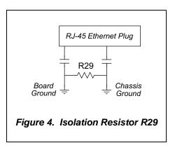
The RJ-45 connector is shielded to minimize EMI effects to/from the Ethernet signals. Z-World recommends that an equivalent RJ-45 connector be used on the user board if the customer wishes to have an RJ-45 connector on the user board.
