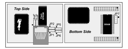
Figure A-5. Location of RCM2200 Configurable Positions
