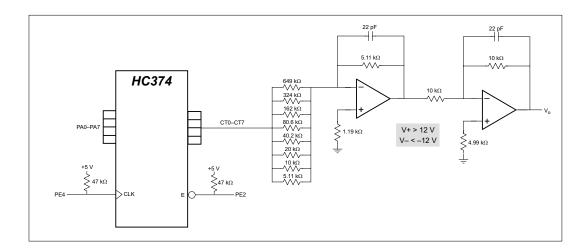
Figure D-5. Sample D/A Converter Connections
