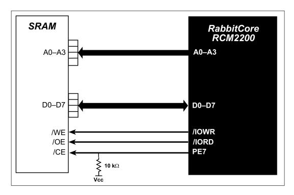
Figure D-4. Sample External Memory Connections
