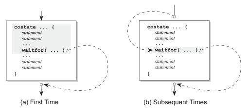
Figure 5-3 shows the execution thread through a costatement when a waitfor evaluates to true.
