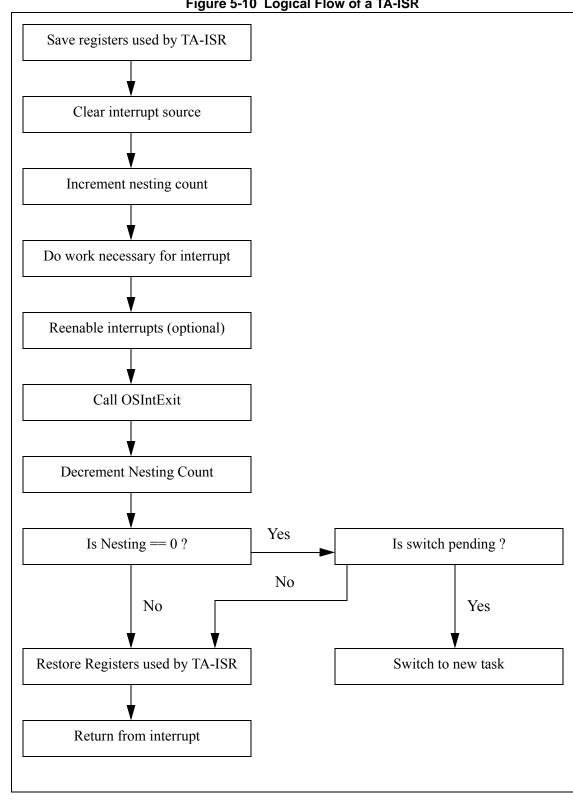
Figure 5-10 Logical Flow of a TA-ISR
