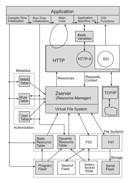
Figure 2.6 Components of a full-featured web-enabled application.
