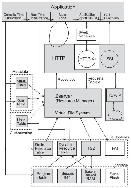
Figure 2.7 Components of a full-featured web-enabled application.
