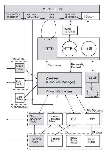
Figure 2.2 Minimum components for a web-enabled application
